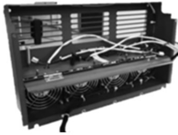
Cooling system module
